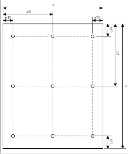
$\text{Uniformity} = \frac{\text{minimum luminance in 9 points (1-9)}}{\text{maximum luminance in 9 points (1-9)}}$ $\text{Luminance} = \frac{\text{Total Luminance of 9 points}}{9}$ |
