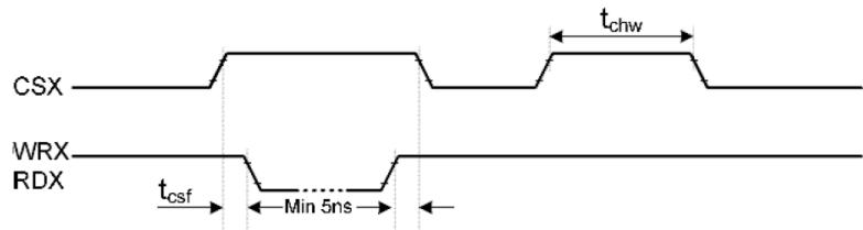
**Note 5:** The Write to Read or the Read to Write timing:
